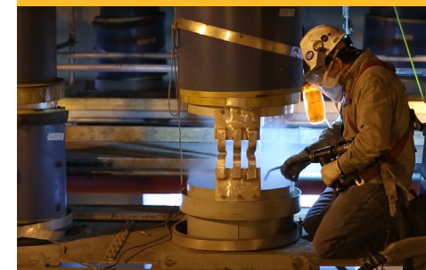
SOLUTION: CRYOGENIC CLEANING
