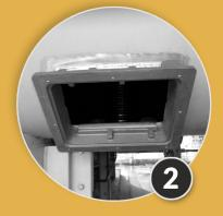
STEP 2 Window base is welded into the enclosure
